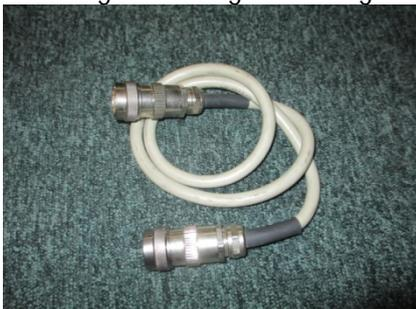
When linking controllers, the analog extension lead must be connected to the "OUT" connector of the first controller and the "IN" connector of the second controller. The last controller in the chain must have the following end plug:
